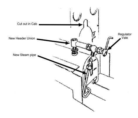
**Operation**: The original forward and reverse valve is now used solely for forward, off, and reverse control. The new cab mounted regulator is now used for control of power and speed, with off being clockwise and open being anticlockwise.
